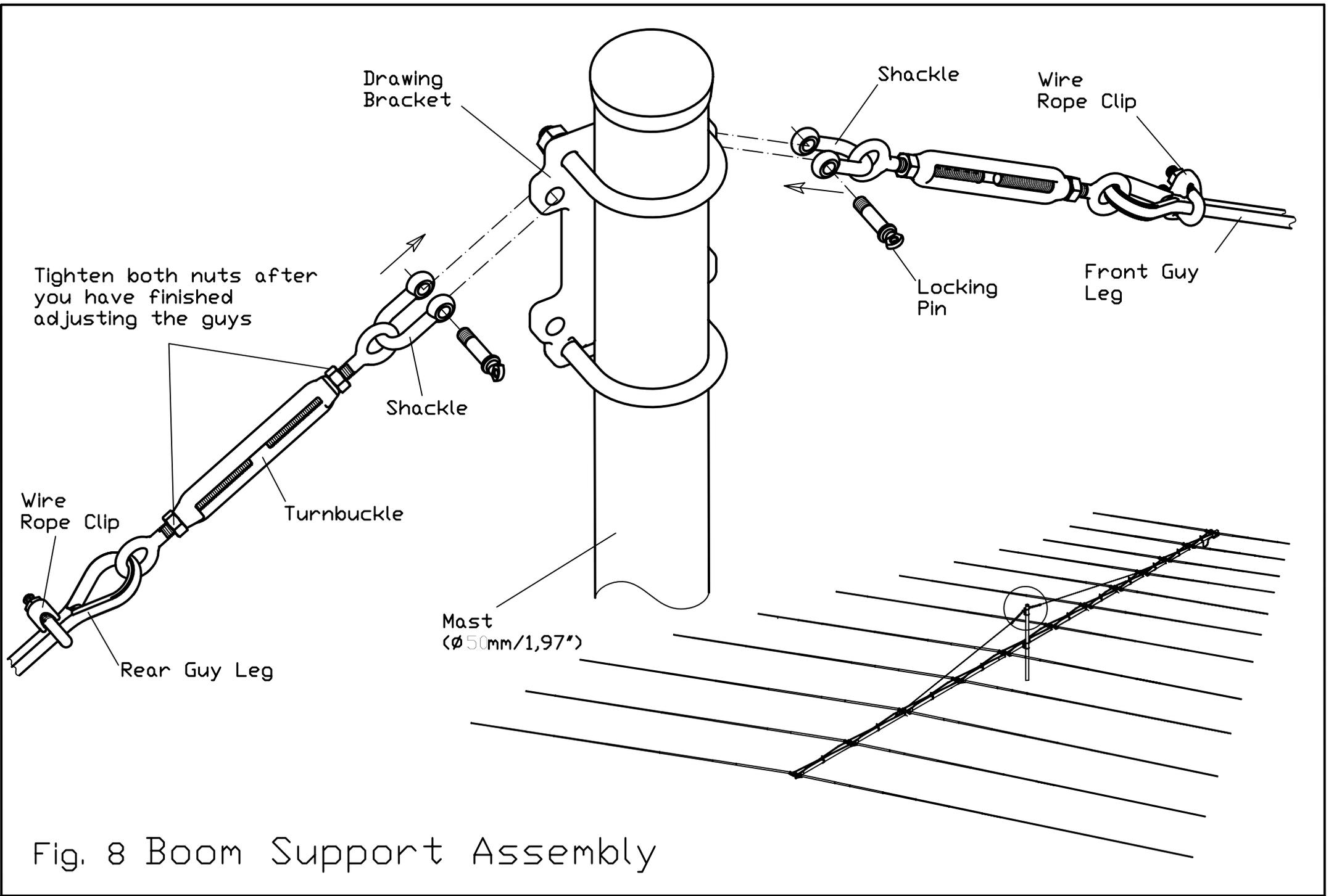
Fig. 8 Boom Support Assembly
