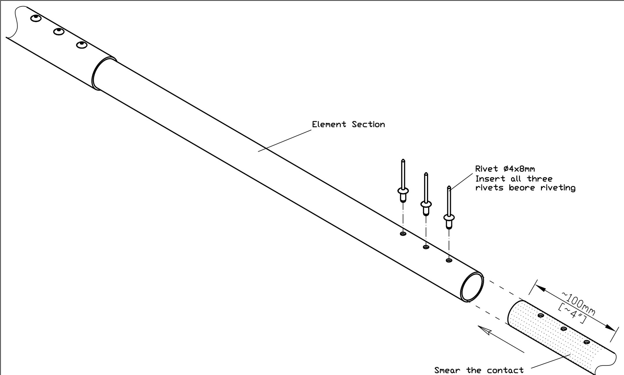
Fig. 3 Element riveting
