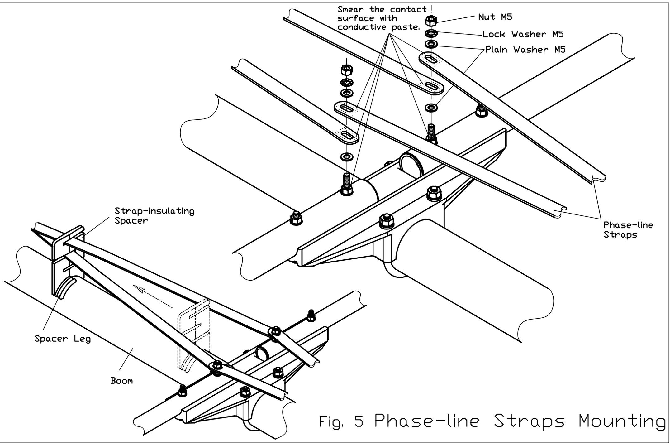
Fig. 5 Phase-line Straps Mounting
